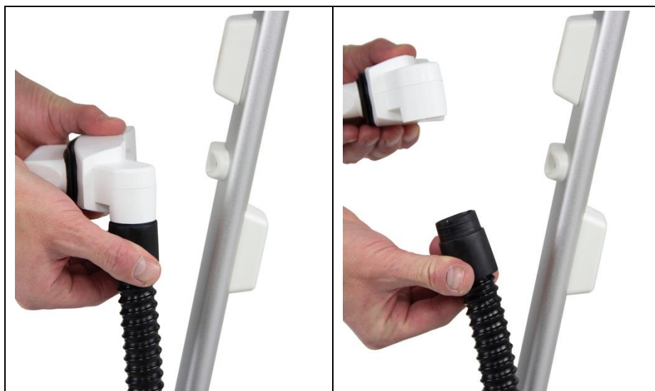
Figure 24: Removing the suction hose waste water
