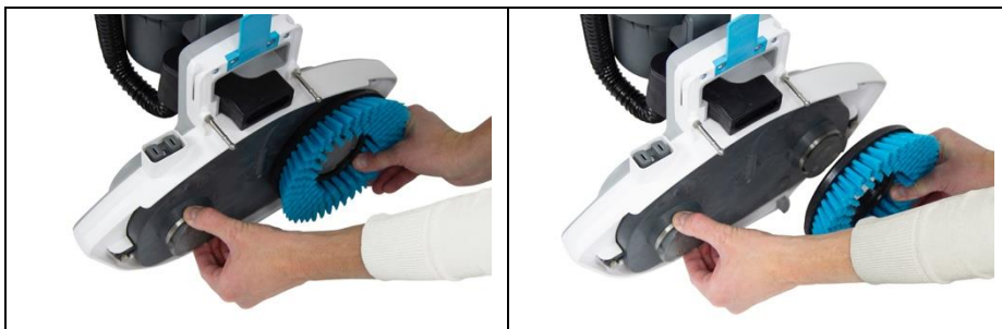
Figure 23: Removing cleaning brushes
