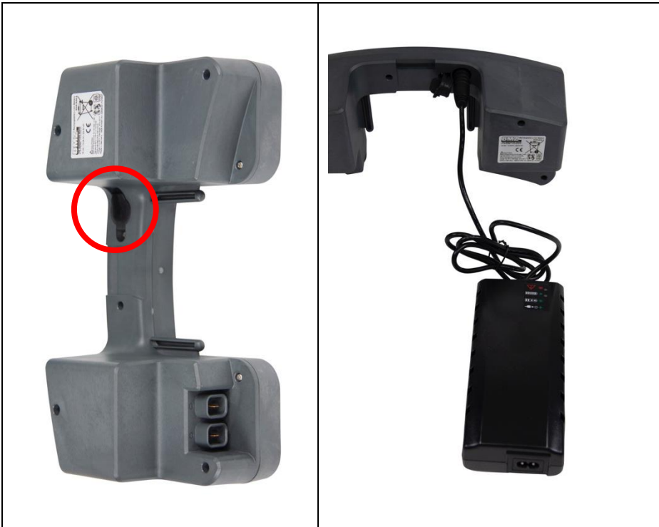
Figure 13: Charging connector on the battery
